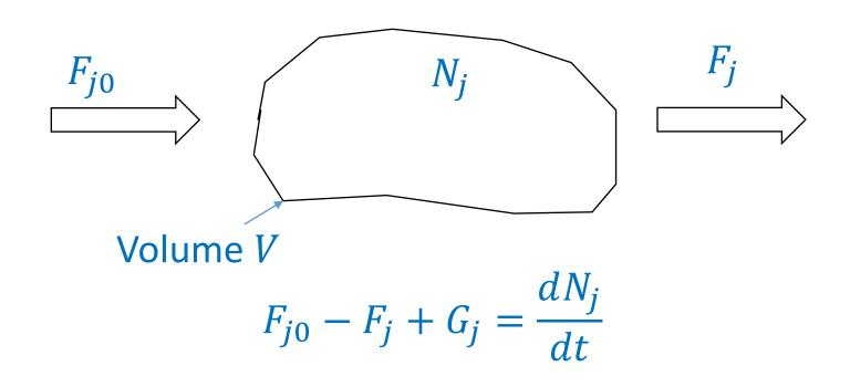
$N_j$  is the # of moles of species j in volume V at a given time  $F_{j0}$  is the # of moles of species j flowing IN per unit time  $F_j$  is the # of moles of species j flowing OUT per unit time  $G_j$  is net generation of species j in volume V per unit time
