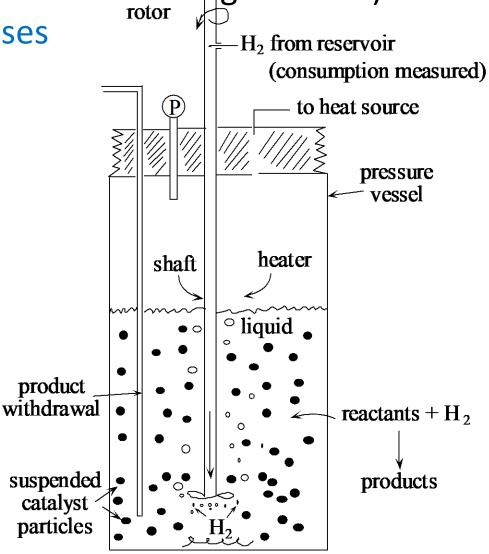
Batch-slurry reactor for hydrogenation of specialty chemicals.
